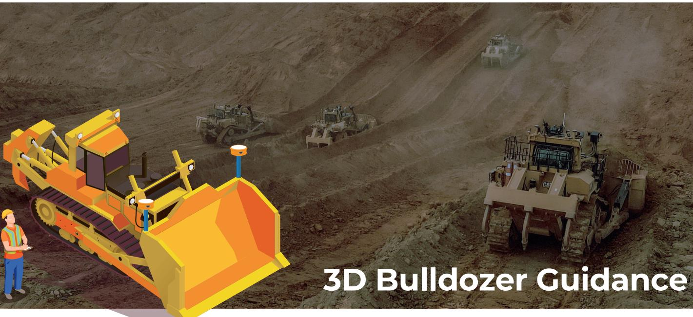
The SITENAV 3D machine control system enables you to tackle any project, whether simple or complex, with centimeter-level accuracy of  $\pm 2$  cm required. From stripping and leveling to ground finishing and earthworks, it boosts your productivity like never before.
